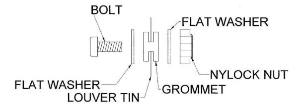
All bolts enter from the outer sides and the nuts from the inner sides.
