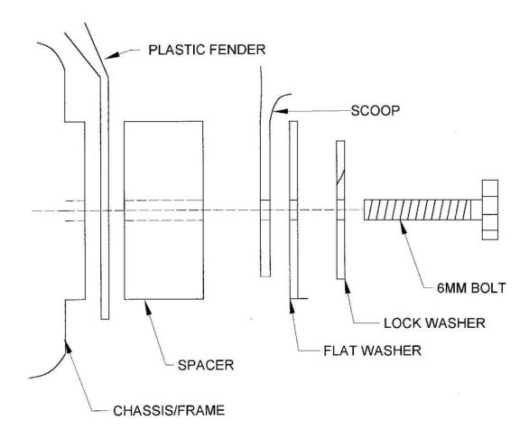
Spacers are used in the upper and lower mounting holes only.
