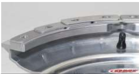
Beadlock shims placed on inner mounting ring
