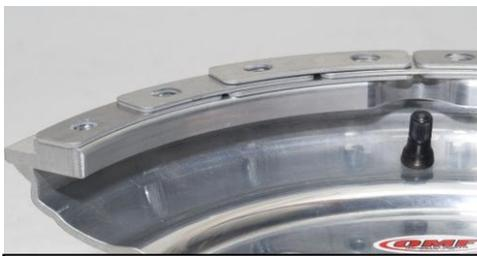
Beadlock shims placed on inner mounting ring
