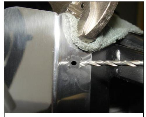
6. Using the drill motor and 1/8" drill bit, drill through existing holes in Gravel Guard and into the frame. Install Tek Screws into these three holes. Do not tighten screws completely, leave slightly loose until step #9.
