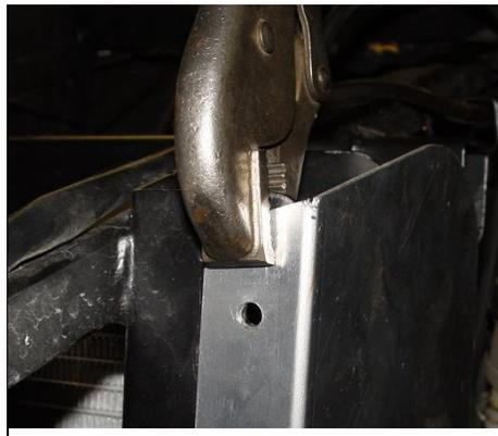
5. Grab drivers side gravel guard and slide it between the shock and shock mount. Align upper part of gravel guard flush with top part of frame near radiator. Use vice grips to clamp gravel guard to frame in position.
