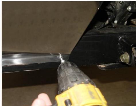
8. Using the 1/8" drill bit, drill one hole through bottom of gravel guard into bottom of frame. Install one Tek Screw. Do not tighten screw completely, leave slightly loose until step #9.
