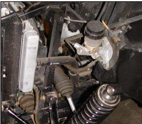
4. Remove upper shock bolt on drivers side using 14mm and 17mm open-end box wrenches. Pull upper part of shock away from upper shock mount.
