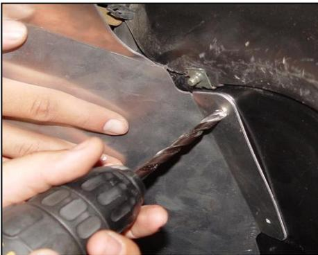
7. For this step, pliers may be needed to "tw eak" the gravel guard rear mounting tab for better fitment. Using the 1/4" drill bit, drill top hole on rear mounting tab through plastic firewall. Install bolt, washers, and nylock nut finger tight.
